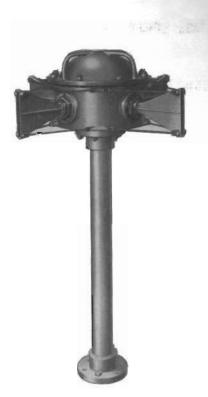
The aerial can be supported on a 3 ft tubular pedestal, (identical to the ANF pedestal) which may be fitted in place of the ANF pedestal or directly on the snort tube, the head of which has been suitably modified. It is orientated on installation so that the horns face Port, Starboard, Fore and Aft, the radiation pattern in the horizontal plane approximating to a cosine law for each horn. Pyrotenax cables feed the video signals to the office equipment.
