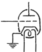
3 ELECTRODE INDIRECTLY HEATED VALVE.
