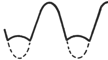
DEMODULATED SIGNAL SEVERE DISTORTION.
