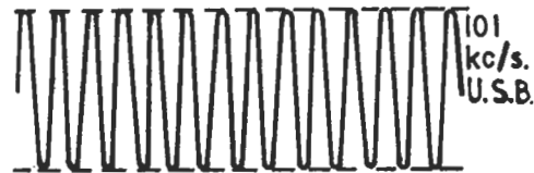
SINGLE TONE OUTPUT AFTER FILTERING OUT THE L.S.B. THIS IS THE S.S.B. SIGNAL THAT IS TO BE TRANSMITTED.
