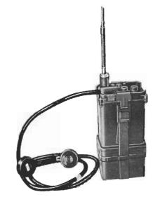
A 13 valve VHF F.M. transceiver, employing plug-in sub-assemblies and circuit stages. The receiver is a GENERAL VIEW superhet., the stages being r.f., mixer, xtal controlled oscillator, 4-double tuned i.f. stages, limiter, discriminator, and a.f. amplifier. The transmitter stages are, P.A., M.O., Ferrite reactor modulator; it is held on frequency by an a.f.c. circuit referred to the receiver crystal oscillator. The set and battery share a common case.
